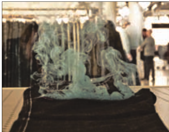
LST Laser is one of several companies using lasers and ozone to "wash" denim without water. Saitex has embraced this technology, and up to 25 percent of its denim is washed entirely without water.
