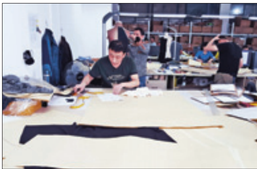
Before: Patternmaking using paper and scissors
