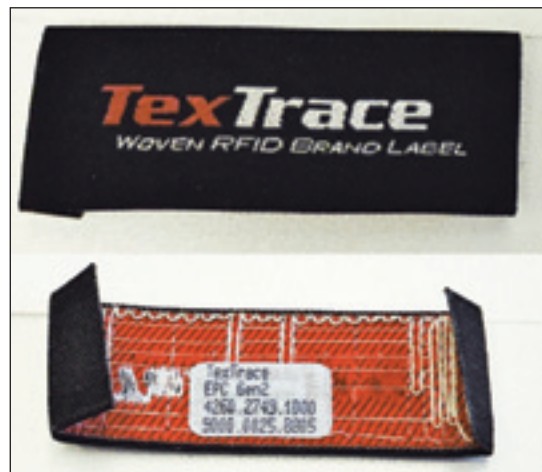
A woven RFID label from TexTrace
