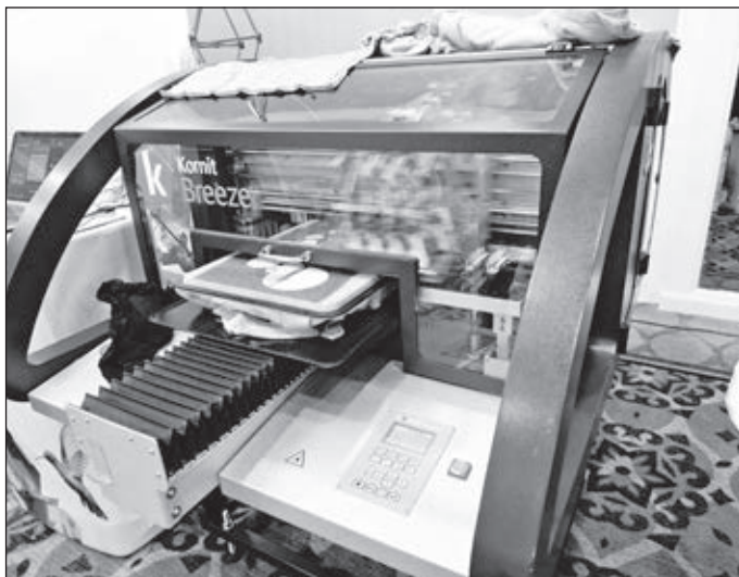
DIRECT-TO-GARMENT: The Kornit Breeze direct-to-garment printer can print up to 50 shirts per hour. Kornit has a larger machine that can print up to 200 shirts per hour as well as a roll-to-roll printer that can print to fabric.
