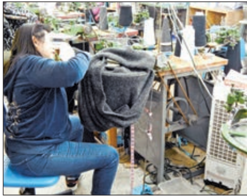
A PDR Knitting employee uses a linking machine to connect the pieces of a project.
