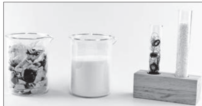
Beakers showing stages of plastic waste (from left): shredded plastic, BioCellection's chemical and threads that could be created from BioCellection's product
