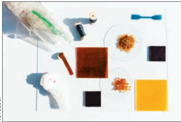
Menlo Park, Calif.’s Novoloop announced on Feb. 23 that it had developed XIRC, a customizable thermoplastic polyurethane material comprising up to 50 percent post-consumer polyethylene waste, which aids in the reduction of trash from single-use plastics.
