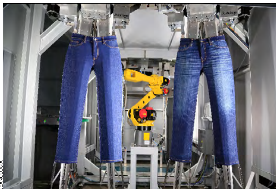
DenimFWD's Urban Factory is home to the first Handman in the U.S. The Handman by Jeanologia automates the laser-technology process and allows one operator to handle the whole production system.
