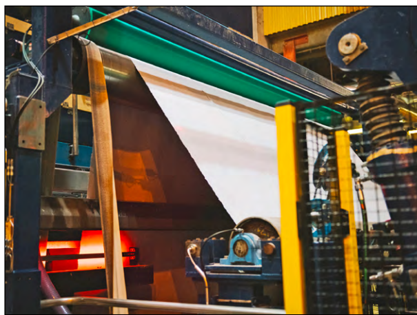
The making of Circulose starts by taking cellulose-rich textiles (right), chopping them up in a shredder, refining them further and using a crusher to make pulp, which looks like big sheets of paper (left). Renewcell then sells the Circulose to fiber producers.
