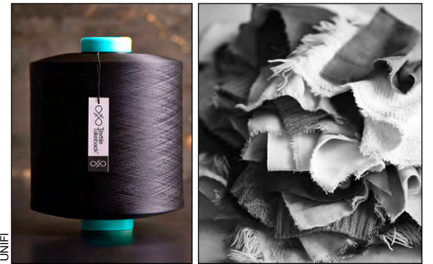
Through a proprietary process, Unifi transforms polyester-based fabric waste (right) into REPREVE fiber (left).
